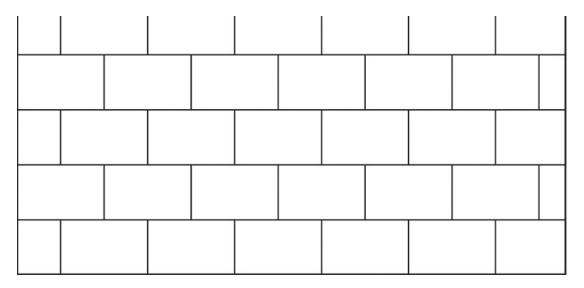
The floor and wall tiles shall be installed using a **"Stretcher Bond" pattern** as shown above. Stretcher bond uses square or rectangular tiles that are laid like bricks in a wall. The end of each tile is lined up with the center of the tiles that are both directly above and below it. This creates a staggered, but cohesive look.
