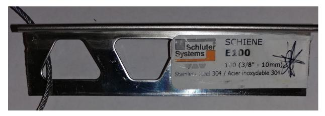
The above picture is of the new wall tile trim and is to be used to cap the 9<sup>th</sup> and last row of wall tile in Camp Bow Wow<sup>®</sup> Luxury Suites and Isolation Rooms. The trim is **series SCHIENE**, **sized 3/8**" **and shall be stainless steel 304** in **nickel finish or anodized aluminum in nickel finish, catalog number E100.** The Camp Bow Wow<sup>®</sup> preferred manufacture is Schluter Systems and the preferred supplier is Daltile.
