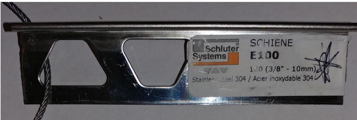
The above picture is of the new wall tile trim and is to be used to cap the 9<sup>th</sup> and last row of wall tile in Camp Bow Wow® Luxury Suites and Isolation Rooms. The trim is **series SCHIENE, sized 3/8”** and shall be **stainless steel 304 in nickel finish or anodized aluminum in nickel finish, catalog number E100**. The Camp Bow Wow® preferred manufacture is Schluter Systems and the preferred supplier is Daltille.
