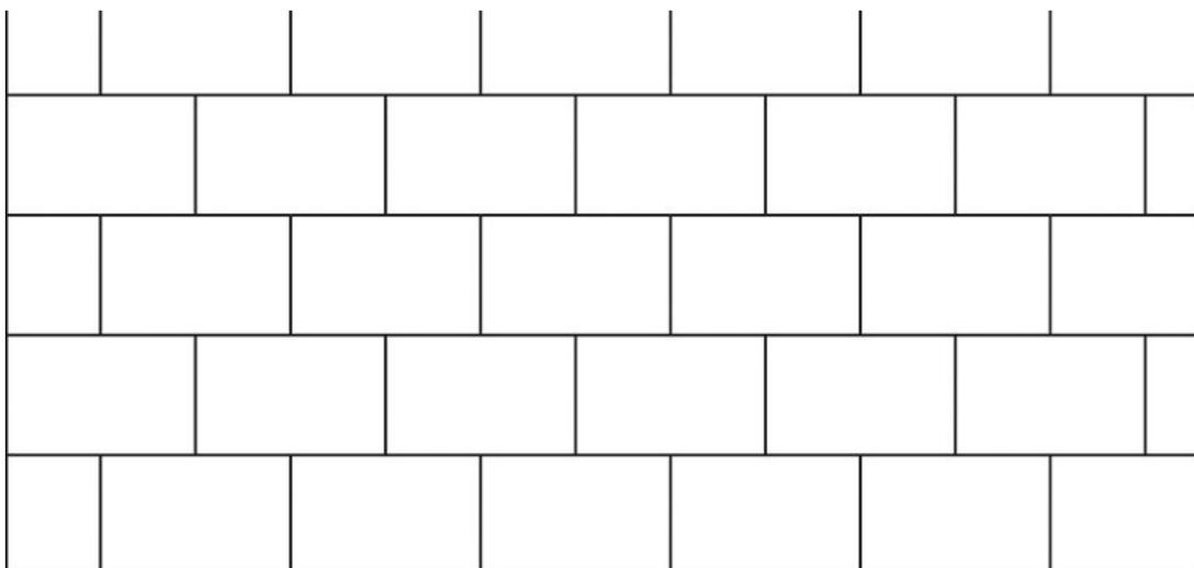
The floor and wall tiles shall be installed using a **“Stretcher Bond” pattern** as shown above. Stretcher bond uses square or rectangular tiles that are laid like bricks in a wall. The end of each tile is lined up with the center of the tiles that are both directly above and below it. This creates a staggered, but cohesive look.
